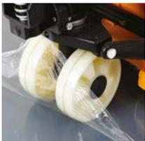
Peel-off mats wrap around the wheels of trolleys and carts. This can create contamination of the cleanroom.
